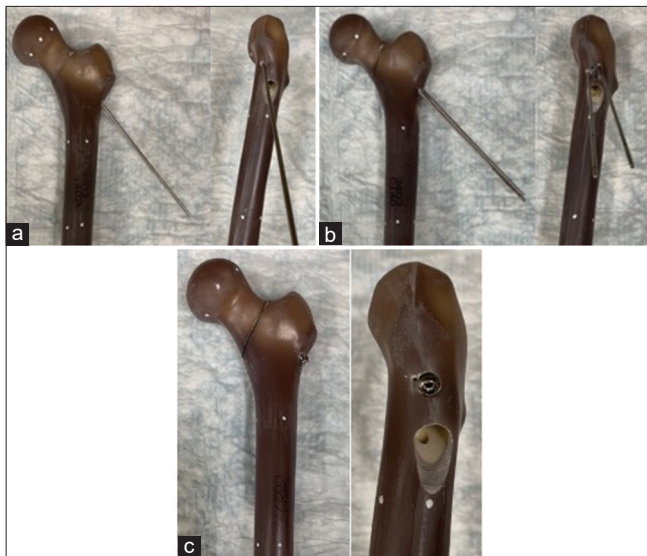
Figure 2: (a) One 2.0 mm K-wire and transcervical-transacetabular K-wire constructs. (b) Two superior 2.0 mm K-wire construct. (c) Single derotation screw construct.
