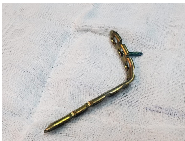
Figure 1: Lateral view of the bent locking plate and jammed locking screw.
